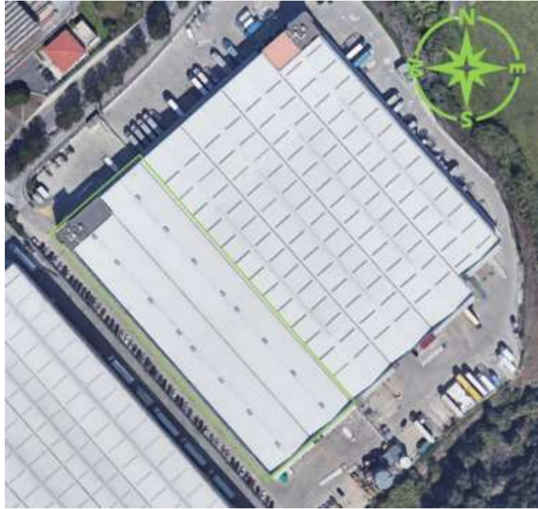
Figure 9: Satellite image of the logistics warehouse, indicating its orientation and the roof space suitable for the installation of solar PV. (Source: Google maps)
